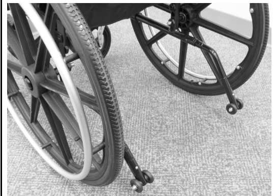
FIGURE 10.2 Changing Orientation of Anti-Tip Wheels
